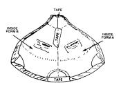
Step (4) Tack solder at least two rows of foiled glass pieces from top to bottom. DO NOT SOLDER GLASS SECTIONS TOGETHER. Bridging pieces will extend from one form to the other. If the glass sections are soldered together by mistake....remelt and separate.
