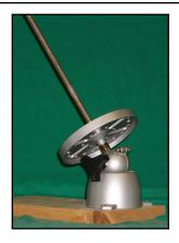
No. 330 is also great for working with partially finished shades whether built on sectional or full forms. Once the vase cap is installed put your lamp on the No. 330 and position the shade to have a level surface for final soldering.
