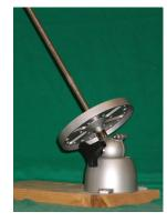
forms. The No. 330 is also great for working with partially finished shades whether built on sectional or full forms. Once the vase cap is installed put your lamp on the No. 330 and position the shade to have a level surface for final soldering.
