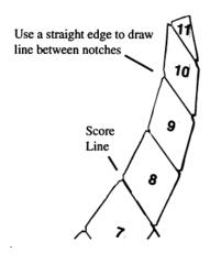
fine marker being sure to mark the notch. Using a straight edge draw a line between the notches. Cut the strip by scoring on the *inside* of your line. Cut the individual parts by scoring in the *middle* of the line drawn between notches. For best fit and color grain flow be sure to keep the parts from each strip in a group. For ease of assembly number each part to keep the parts in order and pieces right side up. The pieces are not square and it is essential to keep the top edge up.
