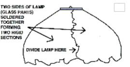
(6) DO NOT BUILD ROUNDED SEAMS ON THE FORM. Remove the lamp and fill and then build the inside seams then do the outside.
