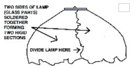
(6) DO NOT BUILD ROUNDED SEAMS ON THE FORM. Remove the lamp and fill and then build the inside seams then do the outside.
