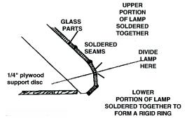
(6) DO NOT BUILD ROUNDED SEAMS ON THE FORM. Remove the lamp and fill and then build the inside seams then do the outside.
