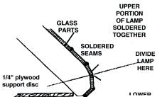
(6) DO NOT BUILD ROUNDED SEAMS ON THE FORM. Remove the lamp and fill and then build the inside seams then do the outside. By filling the inside first, any flow through will be removed when building the outside seams.
