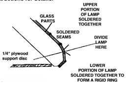
(6) DO NOT BUILD ROUNDED SEAMS ON THE FORM. Remove the lamp and fill and then build the inside seams then do the outside.
