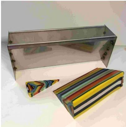
Stainless Steel molds are the most durable mold in the Fusing world. Fiber and ceramic molds can crack with multiple firings but stainless steel can endure unlimited firings.
