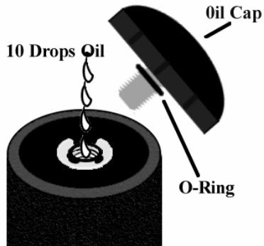
2. Fill the oil reservoir with cutting wheel oil (available at your local stained glass distributor).
