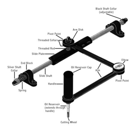
IMPORTANT: The manufacturer has preset the arm for use on a table or bench top. If you are planning to use the Cutter's Mate with the Morton System, you will need to use the grid adapters. It is important for the arm to be parallel to the bench top so that the cutting wheel will remain at a constant 90-degree angle to the glass surface. (See Adjusting Cutter's Mate, but please note that the grid adapters automatically compensate for the change between any flat surface and the Morton System.)
